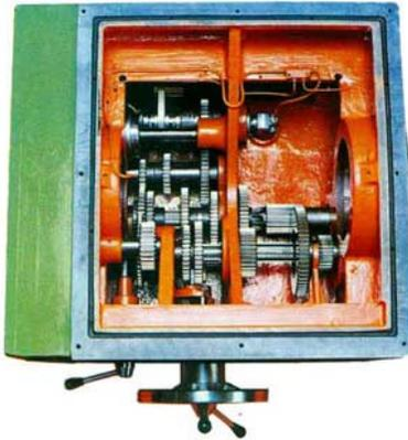
The headstock is a single casting heavily ribbed to give great mechanical strength. The drive and the reverse motion are obtained through a multidisc clutch. On disengaging the clutch an electromagnetic brake automatically disengages the spindle and brings it to rest.
